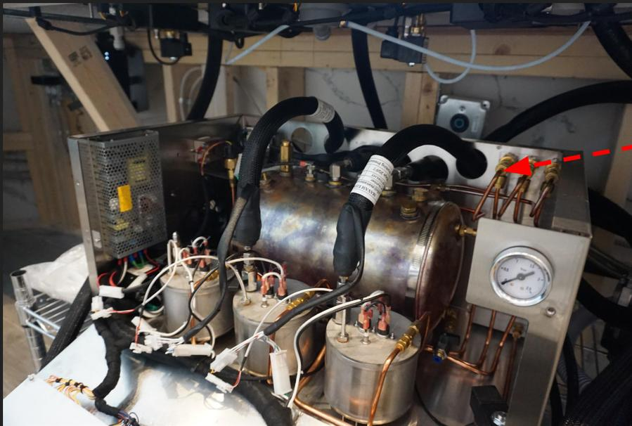
Hoses connected to boilers- center to center, right to right.
